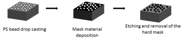
Figure 4.1: Hole-mask colloidal lithography
