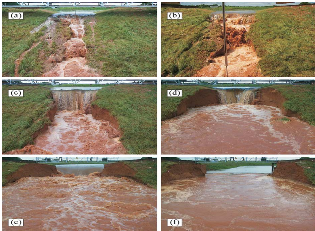
Fig. 6. 22: Phases of cohesive dam breaching by overtopping.
