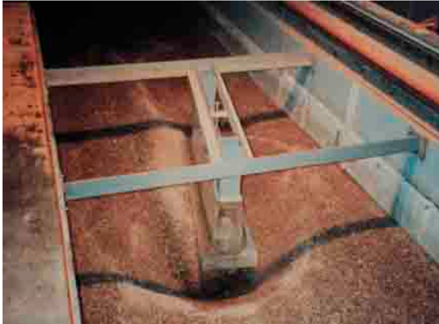
Fig. 6. 64: Physical model represents the scour under bridges.
