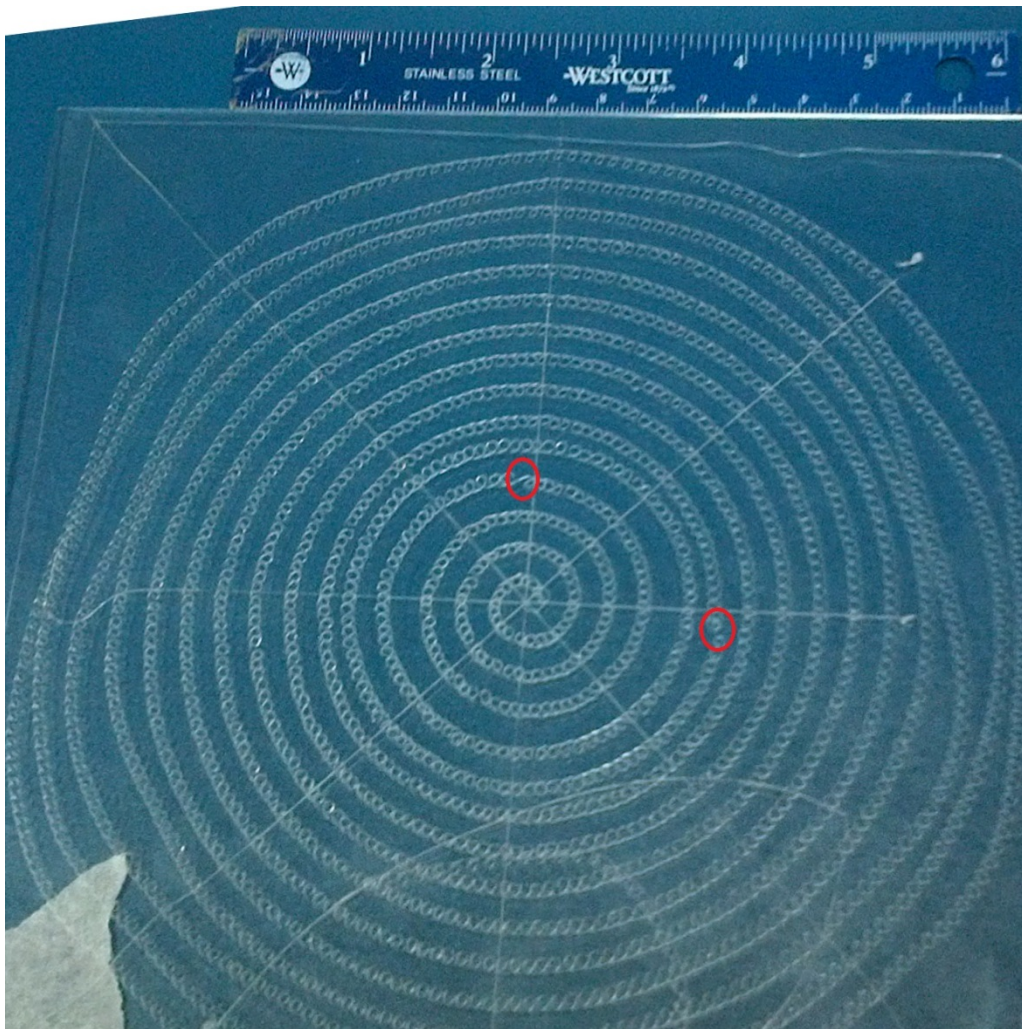
Figure 5-1 A 18 cm diameter web structure deposition attempt, made with a 200\mu\text{m} needle.
