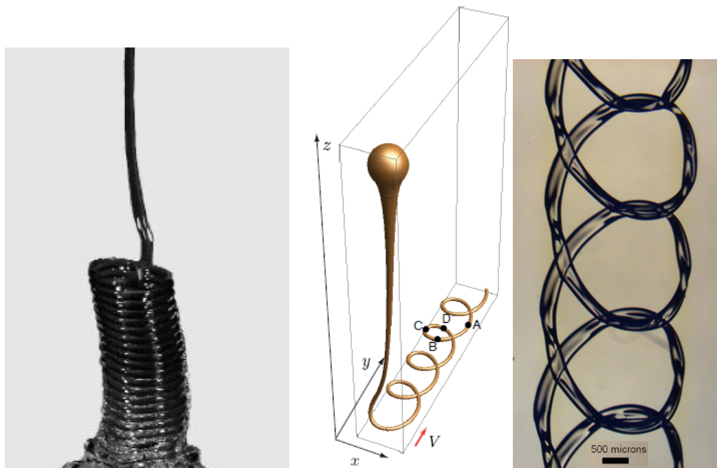
Figure 1-10 Left: example of viscid instability on fixed substrate that produces a coil. Center: viscous instability representation. Right: example of wire realized with a 200 \mu\text{m} diameter of the needle.
