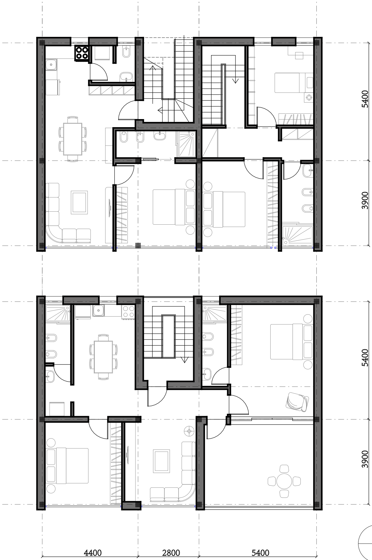
Middle Unit of north-row Plan of First Floor Plan of Second Floor
