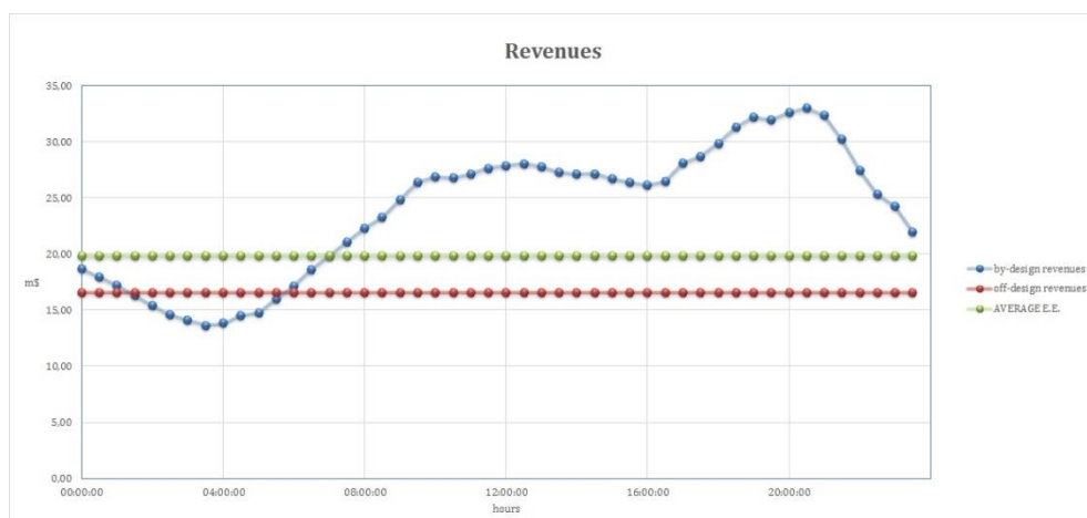
FIGURE 48. DAILY REVENUES FOR THE FIRST DAY OF THE WEEK. IN THIS EXAMPLE THE REVENUES FOR THE OFF-DESIGN CONFIGURATION ARE CALCULATED WITH A WATER PRICE OF 1,2 $/M 3 .
