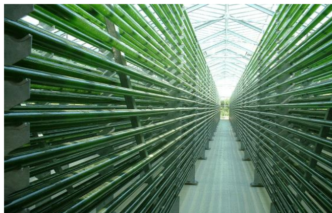
FIGURE 74. THE COMPLEXITY OF THE PBRs. IN PARTICULAR HERE IN THE PICTURE A HORIZONTAL TUBULAR, NATURALLY ILLUMINATED, PHOTOBIOREACTOR SYSTEM.
