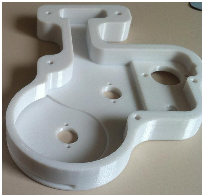
Figure 30: FDM model of the Lateral Arm Support
