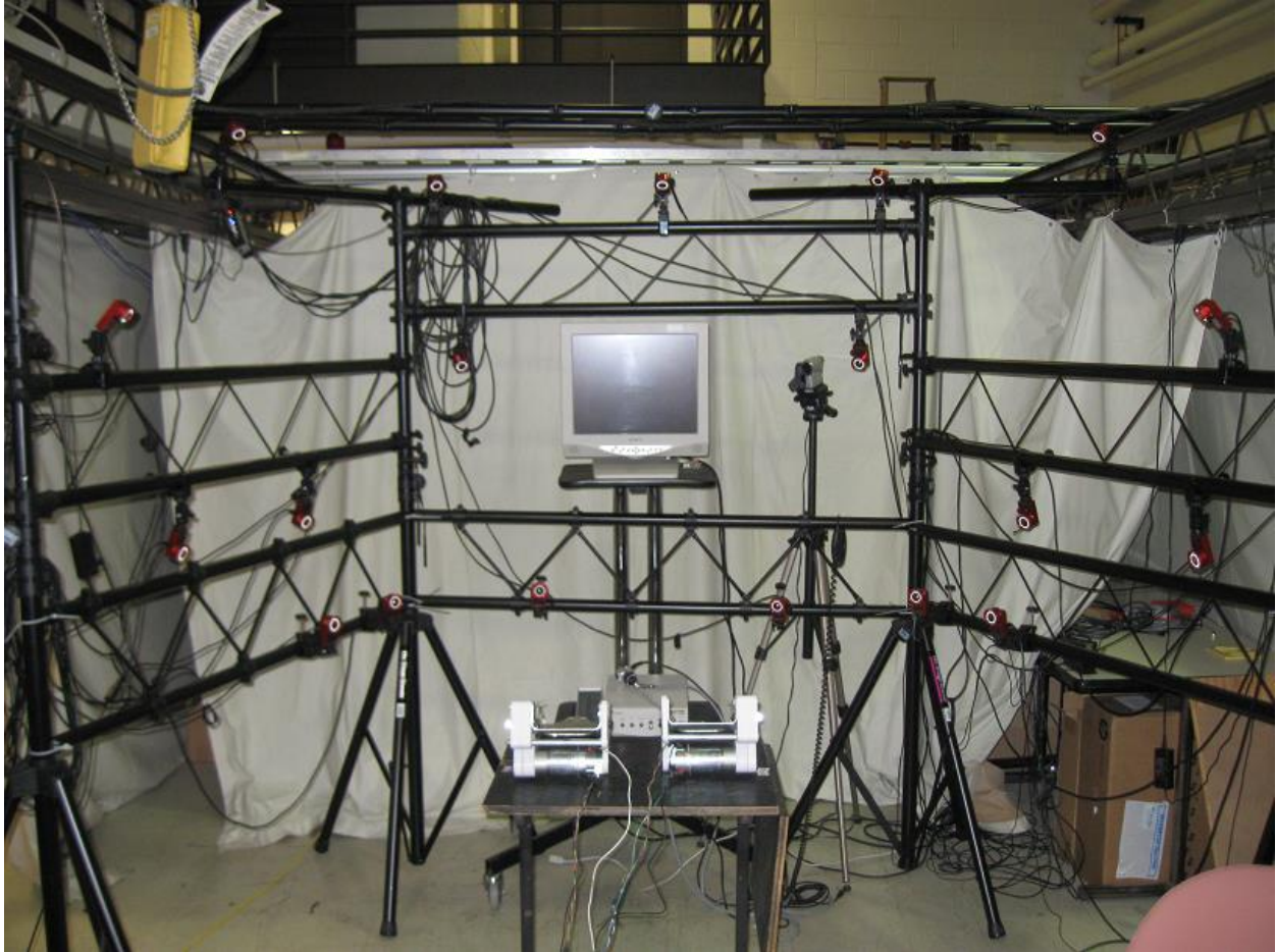
Figure 26: Motion capture setup
