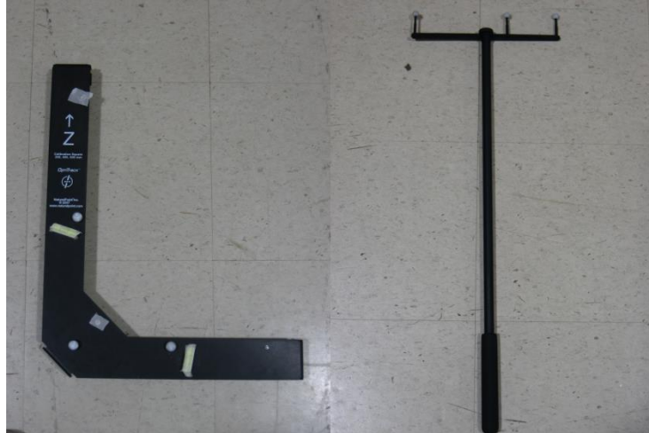
Figure 27: Motion capture calibration square and three marker wand
