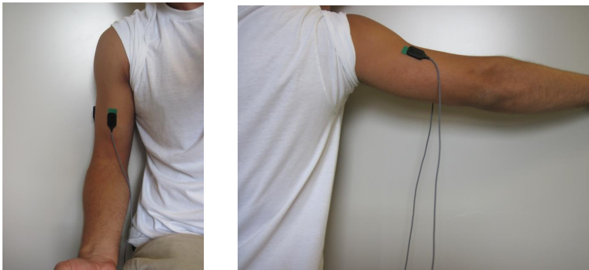
Figure 32: Electrode placement for the bicep (left) and triceps (right)
