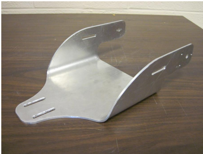
Figure 31: Finalized Aluminum Arm Frames
