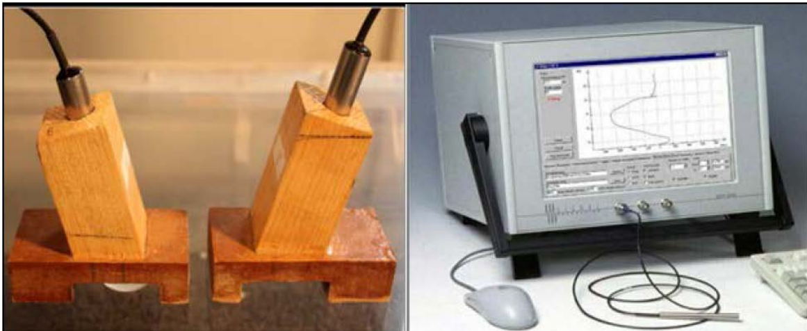
Figure 2.4: Probes position for taking velocity profiles of flow and Doppler 2000.
