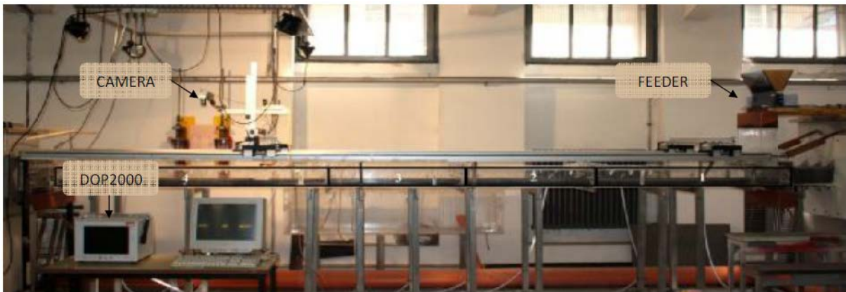
Figure 2.1: Channel configuration at the Hydraulics Laboratory.
