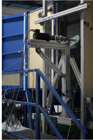
Figure 5.2: The supporting frame and the pitching motor
