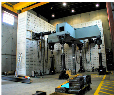
(c) Tavole vibranti (Minnesota and Kassel Universities)
