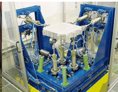
(c) Tavole vibranti (Minnesota and Kassel Universities)
