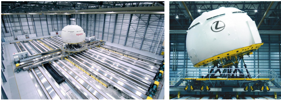
Fig. 1.16: Toyota-Lexus drive simulator.
