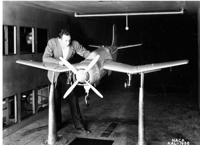
FIGURE 1.5: A scale model of an airplane in a wind tunnel for testing.
