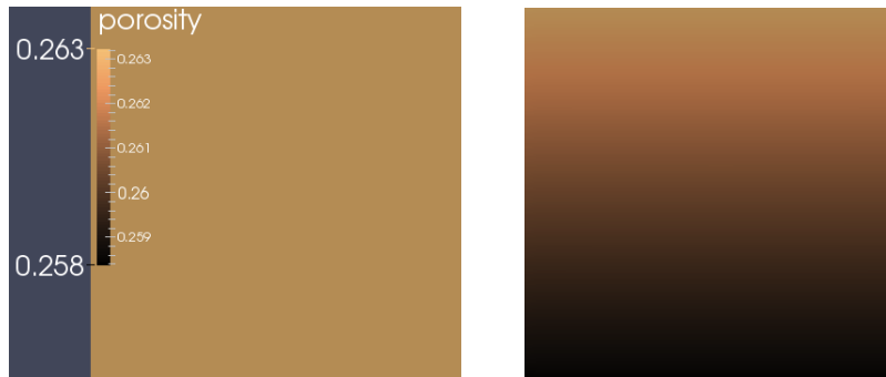
Figure 7: The evolution of porosity \phi . The two snapshots were taken at t = 0 and t = 50 My , i.e. at the beginning and at the end of the simulation.
