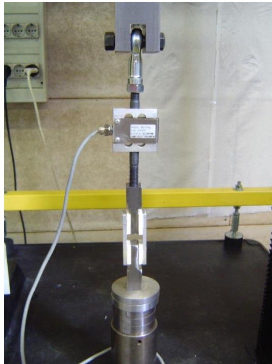
Figure 4.5 The system for pure shear test.
