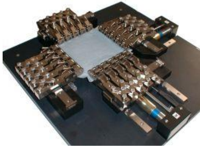
Figure 4.11 The scheme of equibiaxial tension test, adapted from Baidu pictures.
