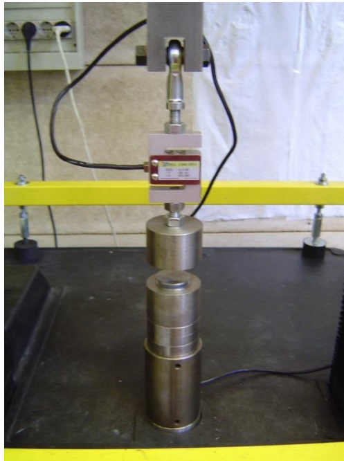
Figure 4.9 The system for compression test.
