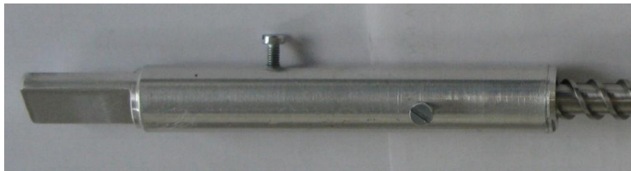
Figure 41 - Holding device for the experiment with the spare drill bit.
