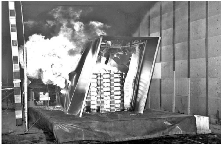
Fig 5-3 Fire experiment with wooden pallets and an aluminum covering carried out in the second Benelux Tunnel, The Netherlands.
