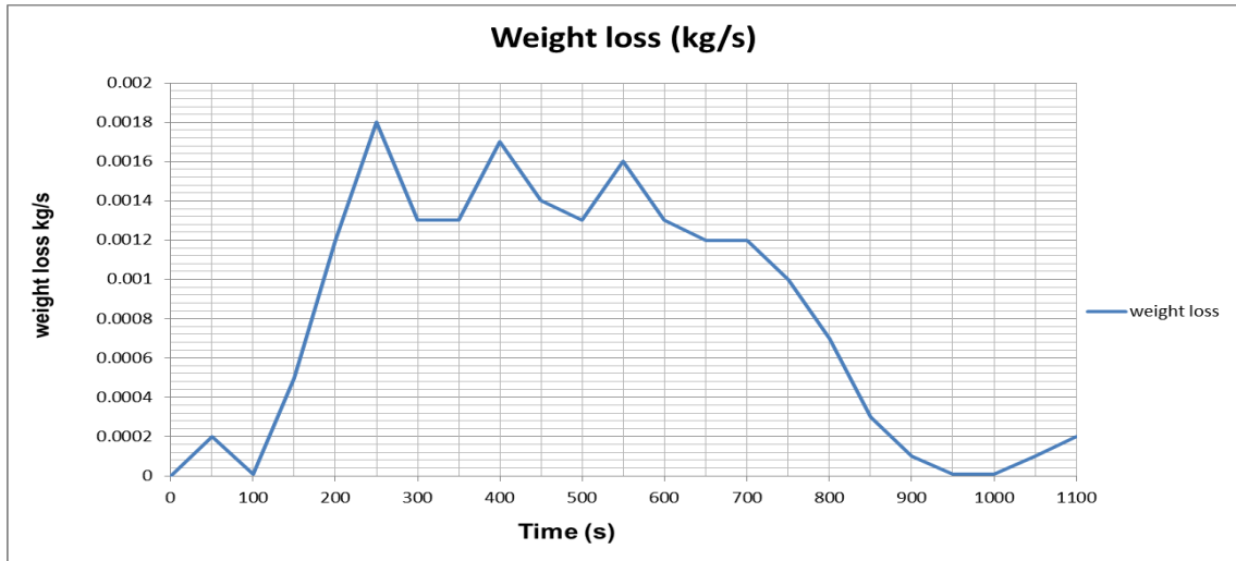
Fig 6-25 Fuel mass loss rate (g) per time (sec) in the third test
