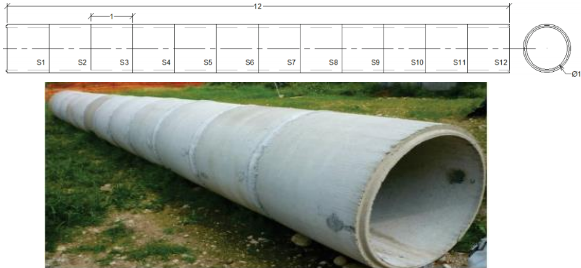
Fig 6-2 Schematic sketch of tube segment arrangement during the test
