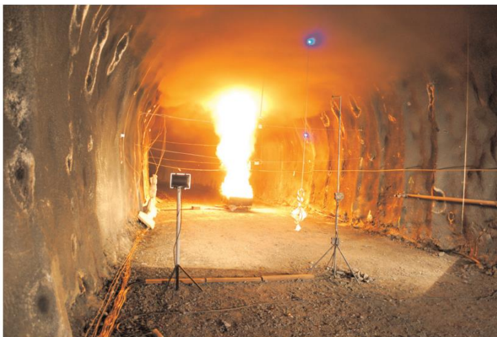
Fig 5-2 Pool fire test in La Ribera del Folgoso Tunnel
