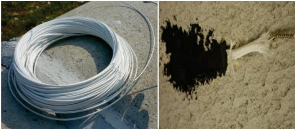
Fig 6-4 Thermocouples and the way of fixation
