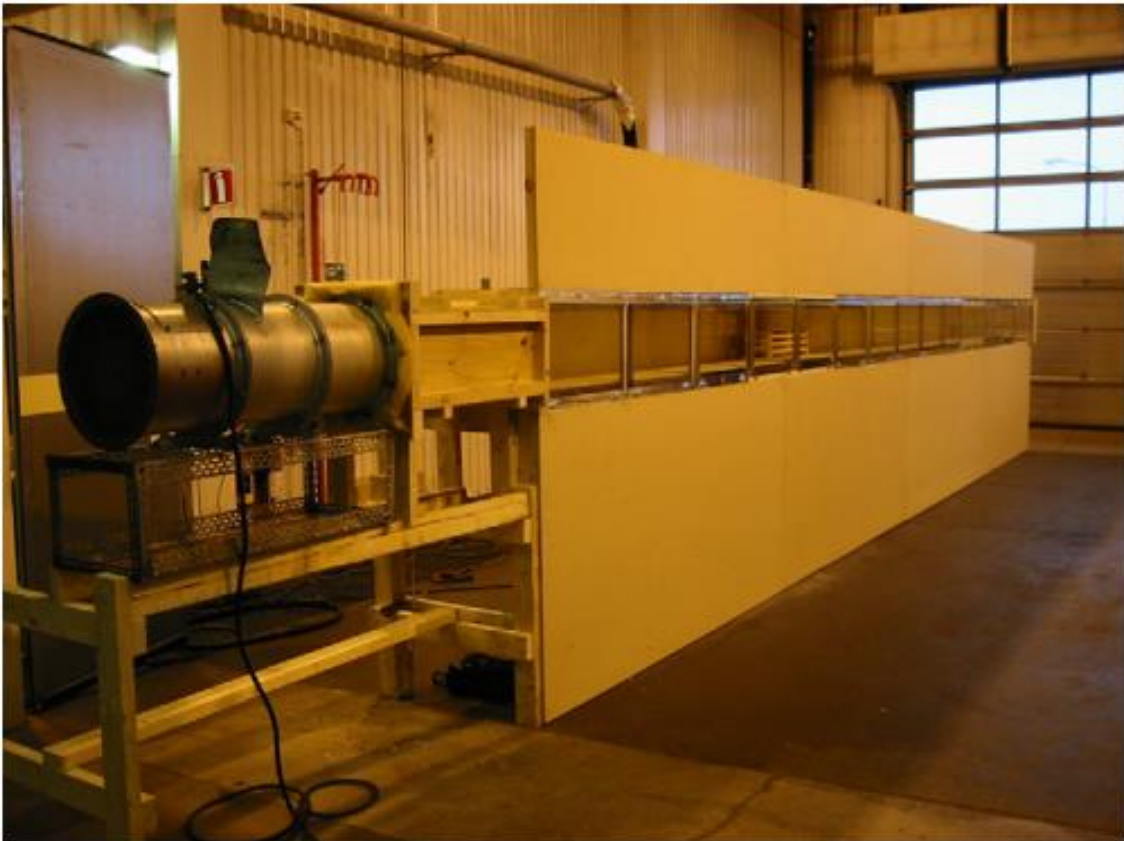
Fig 5-4 A photo of the 1:23 model-scale tunnel
