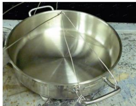
Fig 6-3 Sample of metal fuel container used (with diameter 26 cm and weight 350 g)
