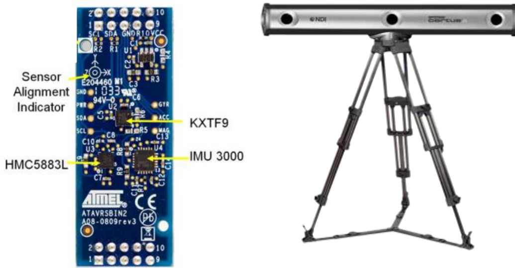
Figure 3.1 Left: Inertial two module from ATMEL. Right: Optotrak Certus Optical tracking system
