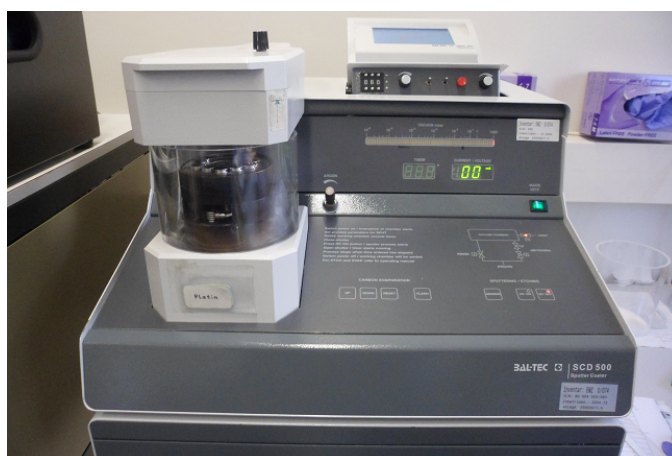
Figure 2.30: Coating of samples in the sputtering machine.
