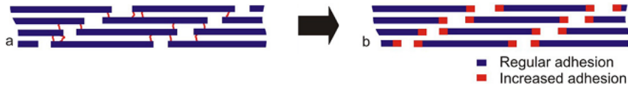
Figure 1.10: Schematic representation of fibril (a) and the model where cross-links are represented increasing the adhesion on the tropocollagen edges (b). Adapted from Buehler Markus J. [23].
