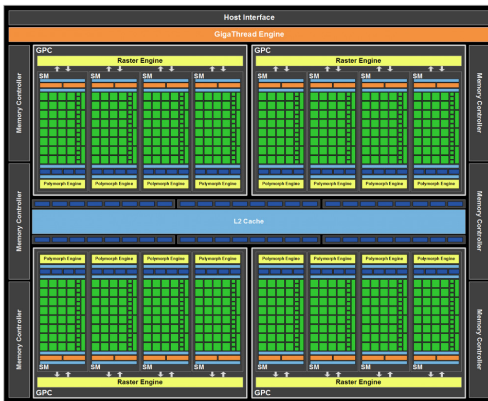
Figure 2.3: Sketch of the NVIDIA GF100 streaming processors array architecture.
