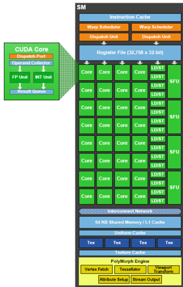
Figure 2.4: Sketch of a multiprocessor on the GF100 gpu, with the new cuda core.
