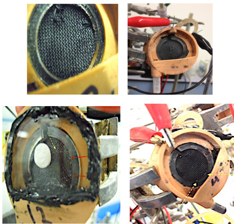
Figure 3.9 - Demonstration of random water drops formation over cathode with different MFCs.
