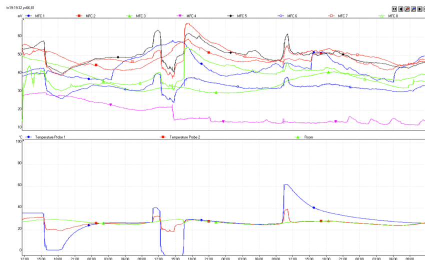
Figure 5.4 - Voltage and Temperature profiles during dynamic temperature sensing experiment.
