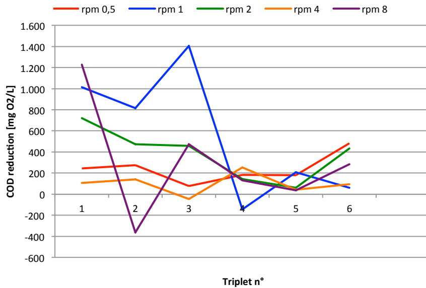
Figure 4.7 - COD reduced by each single triplet at different flow rates.
