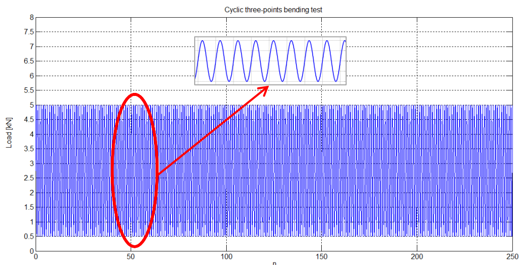
Figure 3.14: Cyclic three-points bending test performed on sample FF_560_3.
