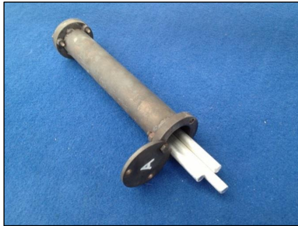
Figure 1.3: Example of precursors inserted in a mold for the production of cylindrical foam samples.
