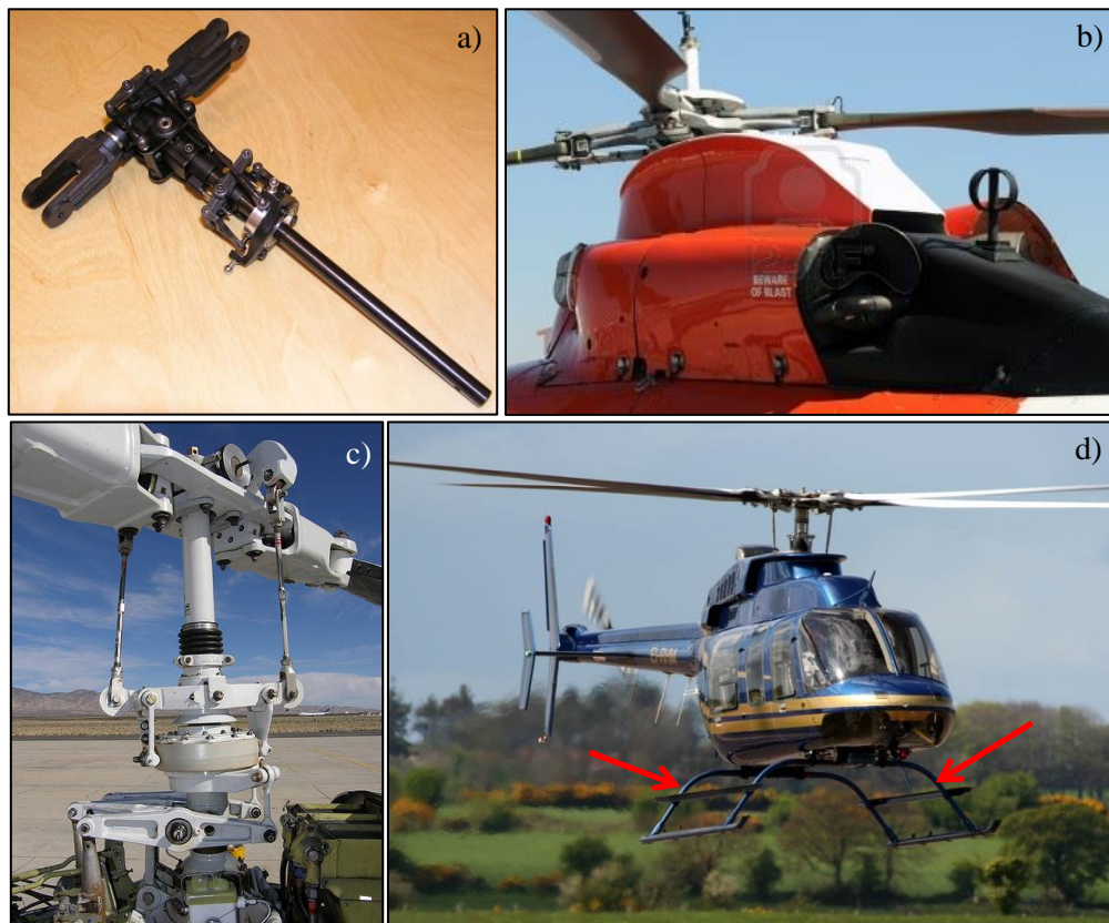
Figure 4.1: a) Preassembled rotor head , b) Detail of an installed rotor and the structure containing the engine, c) Rotor head and flight commands, d) Example of landing gears cross.
