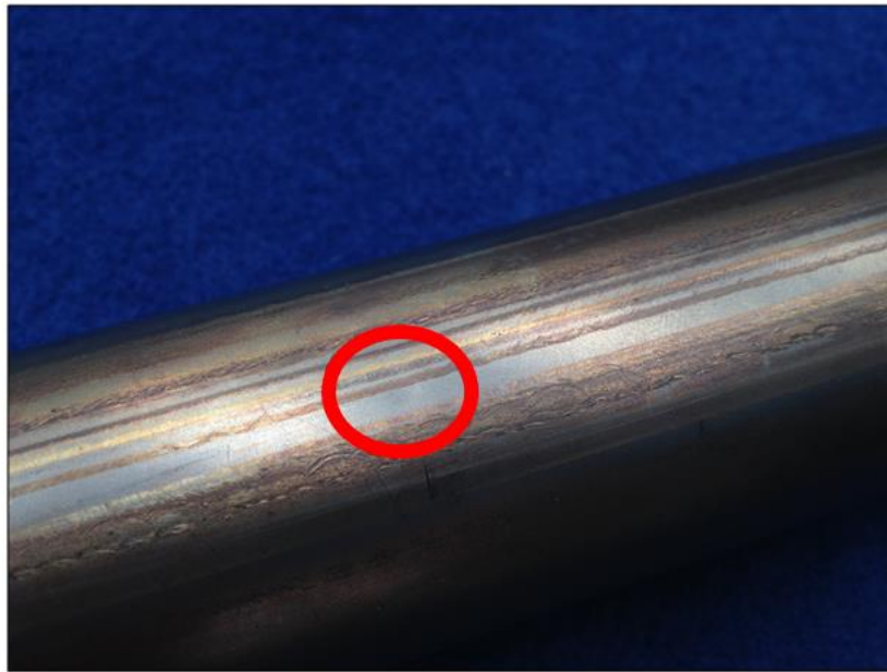
Figure 3.11: Comparison between the plastic deformation in correspondence of the point of contact with the former of samples ET_1 (a) and sample FF_815_1 (b), after the cyclic bending step loading tests.
