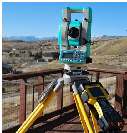
Figura 2.18: Total Station Nikon DTM-652, 500-X data collector.
