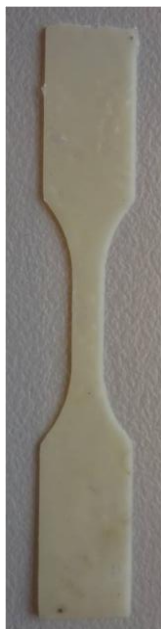
Figure 3.2. Polymeric sample cut according to ASTM D638 regulation
