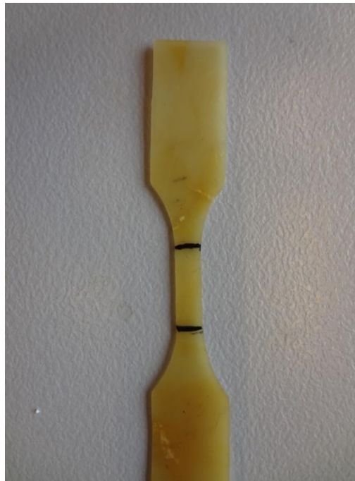
Figure 3.3. Black stripes printed at sample sensitive zone extremities
