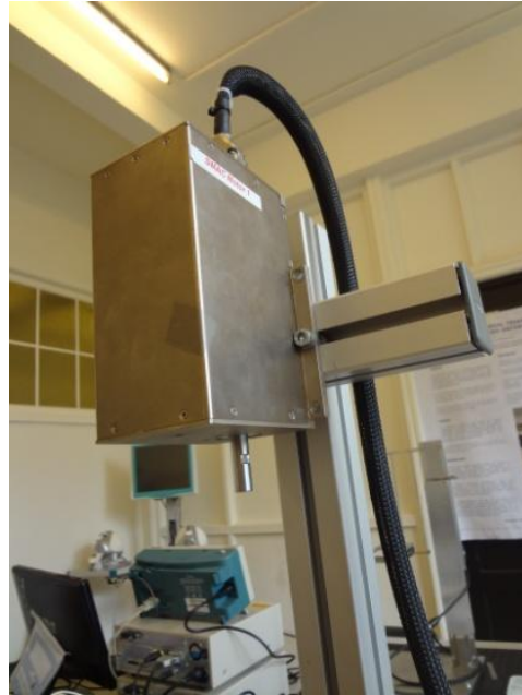
Figure 2.13. SMAC LAL95-050-7; actuator adopted for the assembly of test bench
