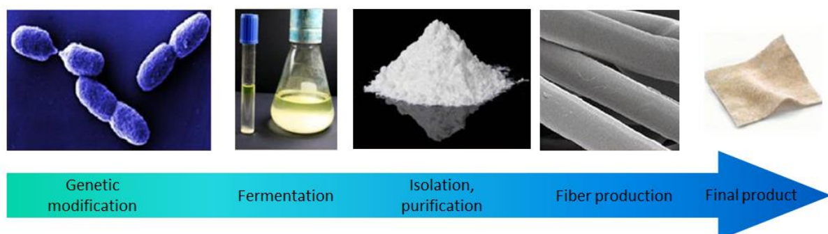
Figure 20: Schematic representation of fiber production from biosynthesised materials
