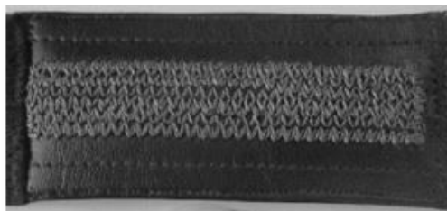
Figure 52: Textile-based electrode for ECG recording
