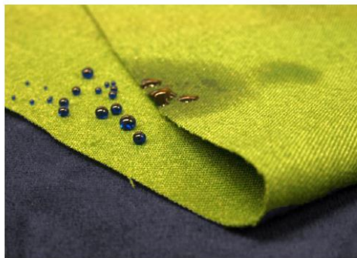
Figure 3: Bifunctional textile obtained by spray finishing
