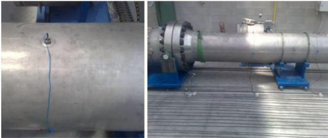
Figure 2.5.4 Pressure transducers on driven section (Corti L., Corti L.G., 2012)
