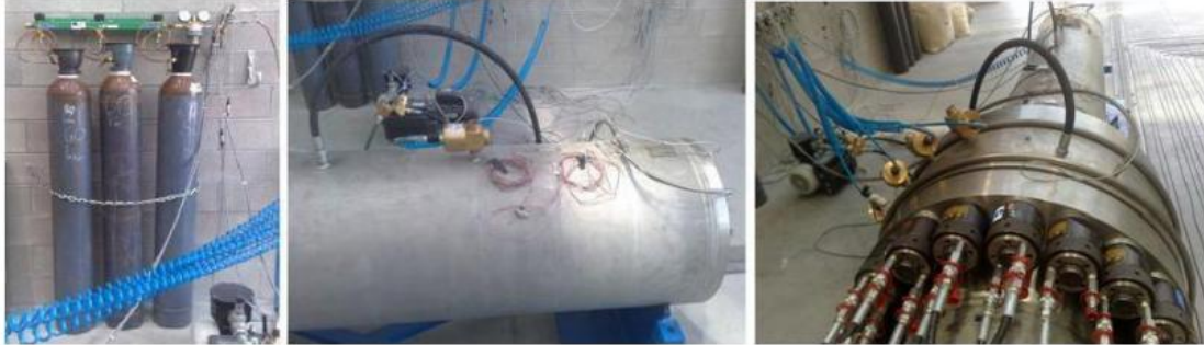
Figure 2.2.9 Helium entering into the chamber buffer and driven (Corti L., Corti L.G., 2012)
