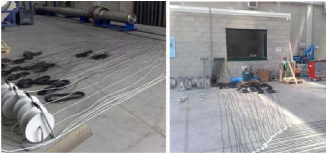
Figure 2.5.10 Cables between the shock tube with the control station (Corti L., Corti L.G., 2012)
