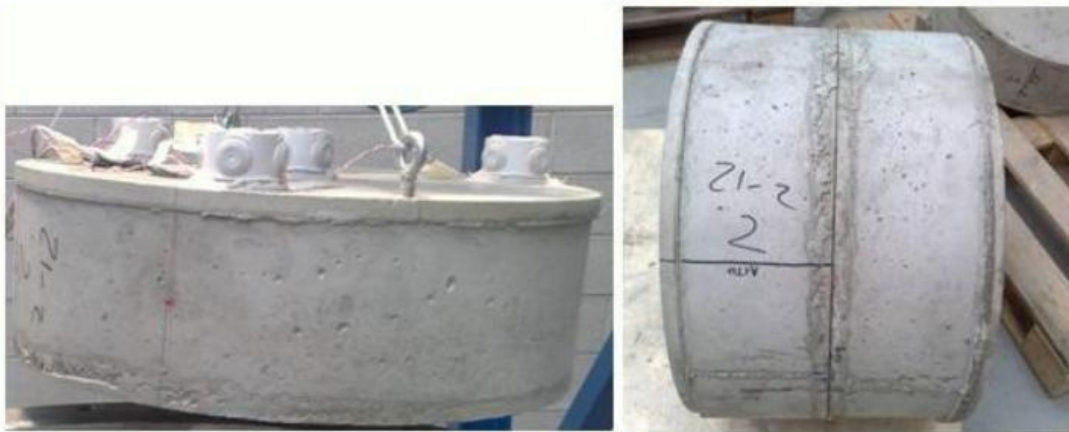
Figure 2.3.1 The specimen composed of three layers (Corti L., Corti L.G., 2012)
