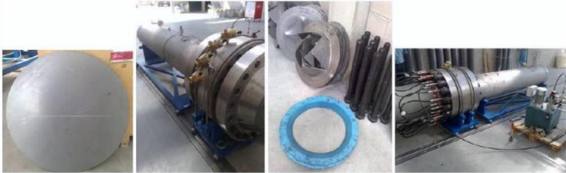
Figure 2.2.1 Steel diaphragm and assembly stage of driver, buffer and driven (Corti L., Corti L.G., 2012)
