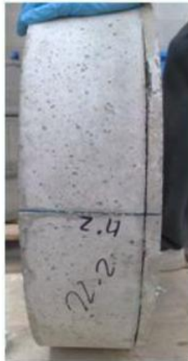
Figure 2.3.2 The specimen composed of two layers (Corti L., Corti L.G., 2012)
