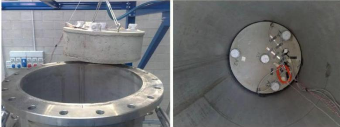
Figure 2.2.2 Positioning of the hard concrete instrumented inside the specimen/soil chamber (Corti L., Corti L.G., 2012)
