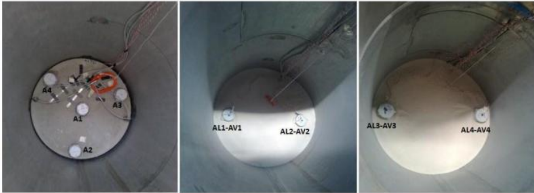
Figure 2.5.9 ICP accelerometers on different sections (Corti L., Corti L.G., 2012)
