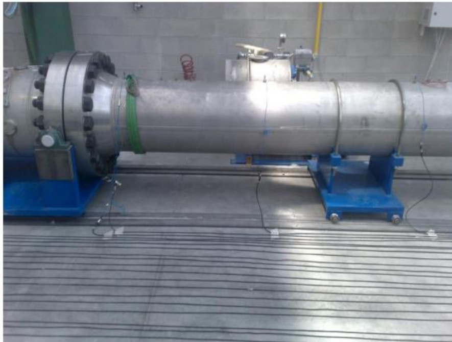
Figure 2.5.1 Position of the dynamic pressure transducers on the driven chamber (Corti L., Corti L.G., 2012)
