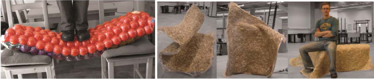
33 Una semplice struttura vacuumatics provata da Frank Huijben (Fonte: F. Huijben, "Vacuumatic Prestressed Flexible Architectural Structures", 2007) 34 Una struttura fine vacuumatics provata da Frank Huijben (Fonte: F. Huijben, "Vacuumatics shaping space by freezing the geometry of structures", 2007)
