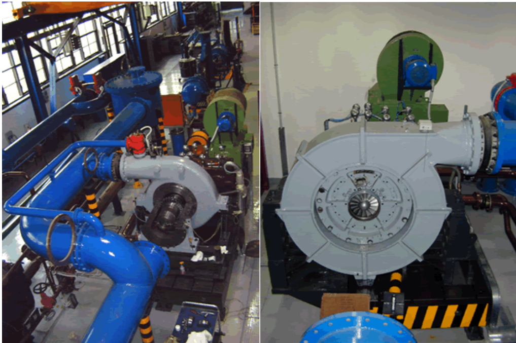
Figure 3.2 Axial and Centrifugal Sections of the Test Rig
