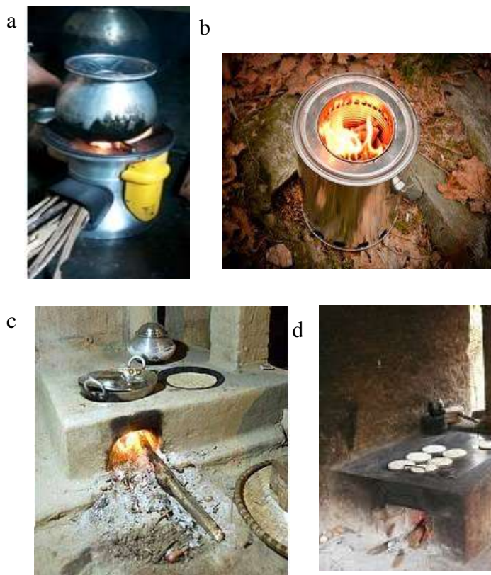
Fig 3.2 (a)Thermoelectric fan stove. (b) Gasification stove. (c) Multiple burners. (d) Griddle stove
