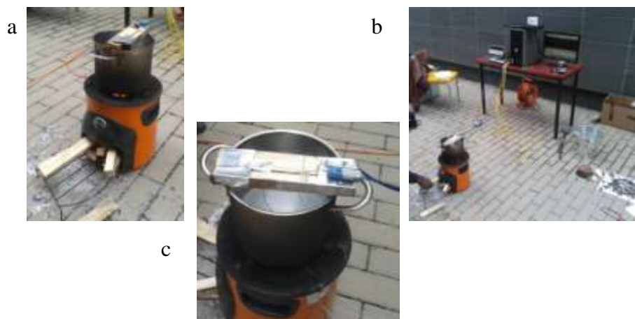
Fig 4.1 Envirofit 3300 (a) Experiments equipment (b). Simply system to handle the thermocouple
