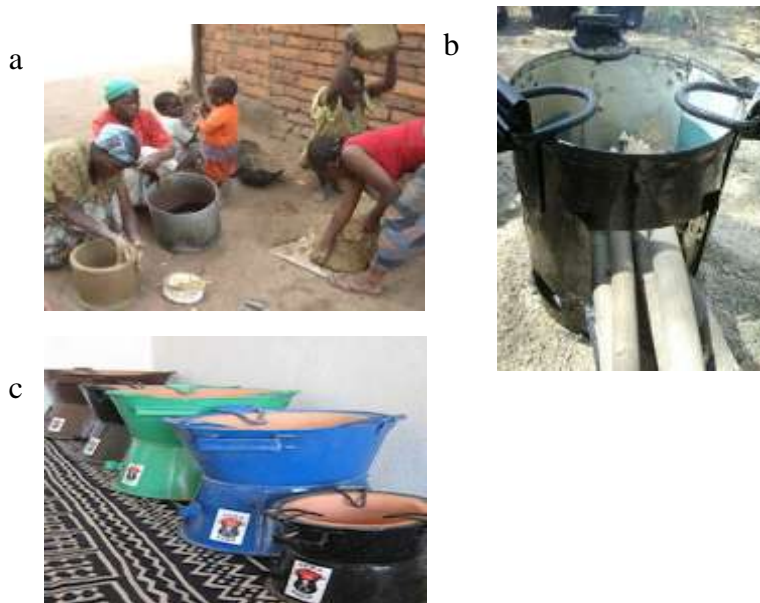
Fig 3.1 (a) Stoves built in place. (b) Side feed stove. (c) Stoves with ceramic lined
