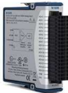
Figure 5.13: Voltage Input Module NI9205
