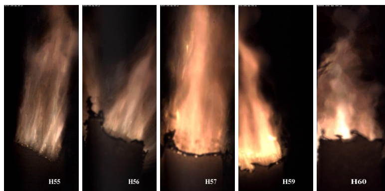
Fig. 5.2. Burning of ADN/GAP propellants at 4 MPa
