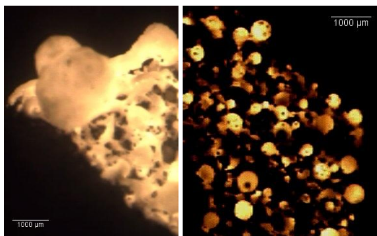
Fig. 5.38. Skeleton layer observed for propellant H54 (left) and H53 (right) at 0.1 MPa.
