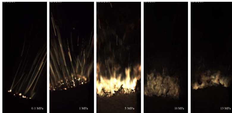
Fig. 5.54. Burning behaviour of propellant A6
