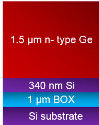
Figure 4.4: Schematic view of the sample with detailed epitaxial steps.
