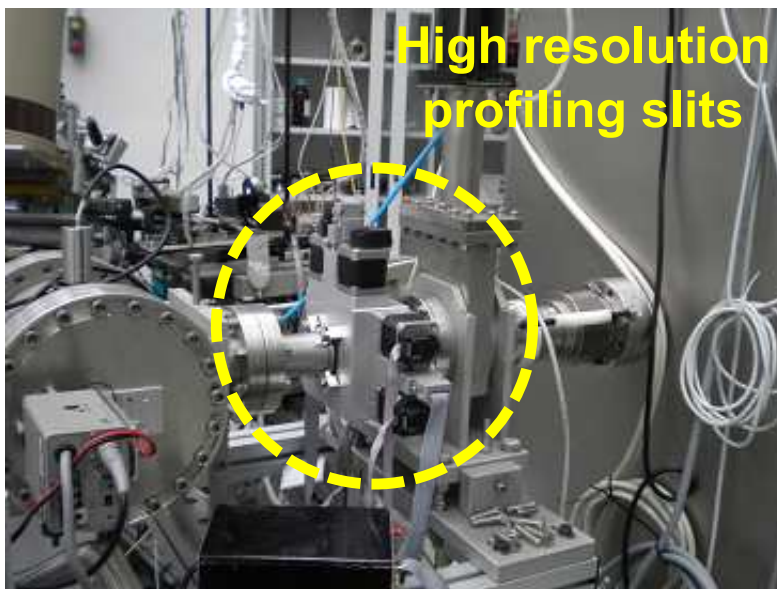
Figure 2.12: The new in-vacuum high-resolution beam profiling slits installed at the DE-FEL beam line (here showed the final slit n°3).
