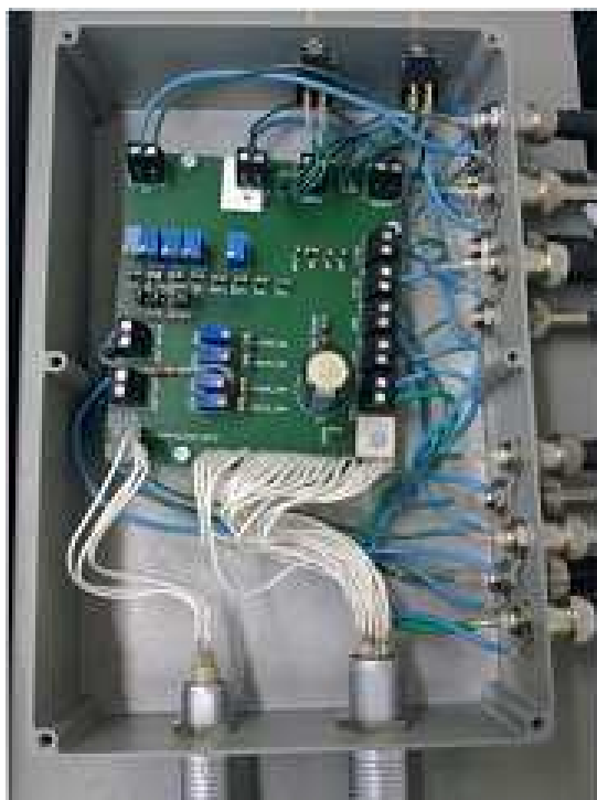
Figure 4.12: The POWER BOARD, responsible for the generation and control of all the DC voltage levels required for the operation of the detector and of the readout electronics.
