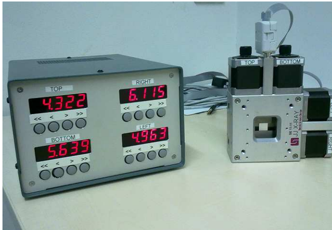
Figure 2.21: Photo of the controller and the profiling slit (in-air version, JJ X-ray IB-C30-AIR model).
