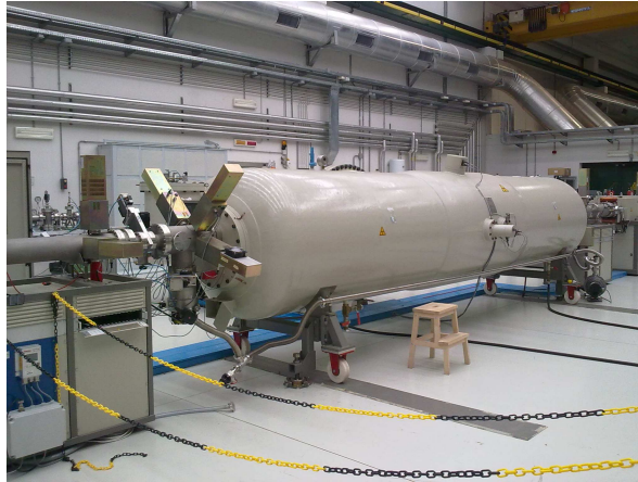
Figure 2.4: The 3 MeV Tandetron ion accelerator system (of the tandem type) at LABEC, produced by High Voltage Engineering Europa B.V.
