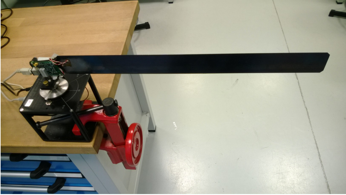
Figure 4.1: Experimental setup of a single link flexible manipulator
