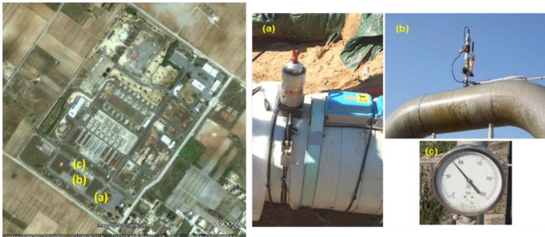
Figure 6.4. Satellite view: TMPC TRANSMED station of Mazara del Vallo (Italy) and sensor location.
