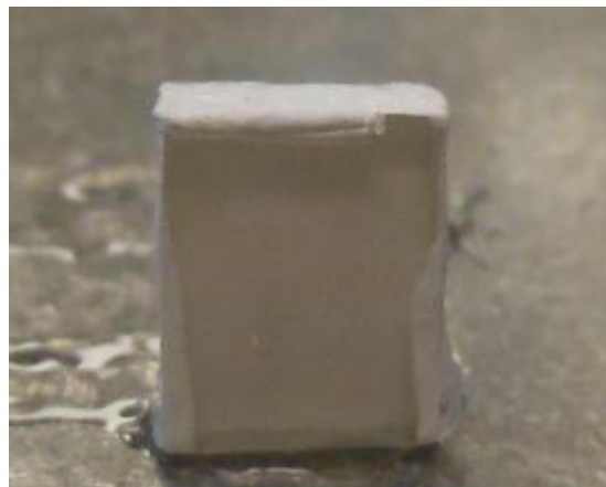
Fig.III.3: A sample of the BC-404 scintillator –based converter covered with BC-620 reflective paint.
