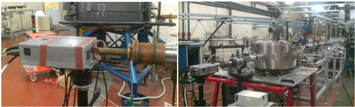
Fig.VI.8: Setup of the ACSpect at LNL: the spectrometer and the Be target (left); the beamline (right).
