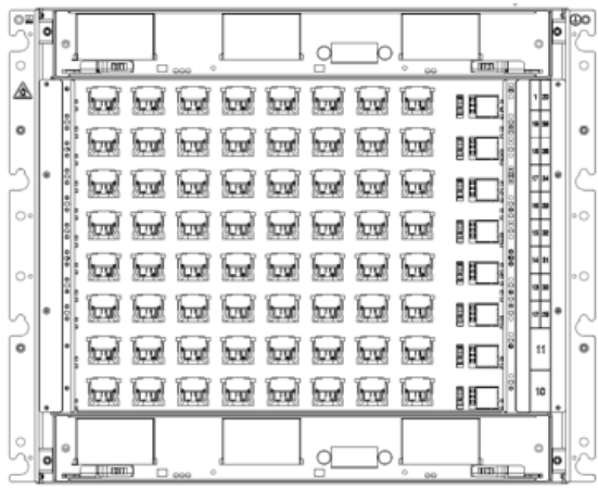
Figure 2.22: Hypothesis of final backplane layout.
