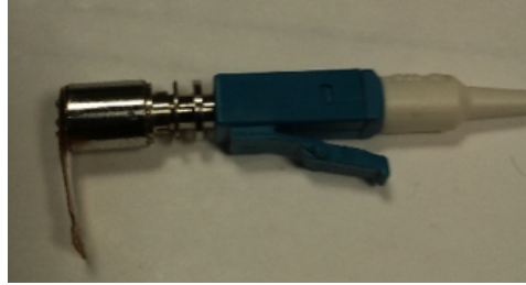
Figure 2.30: Raycan pigtailed VCSEL with LC connector.
