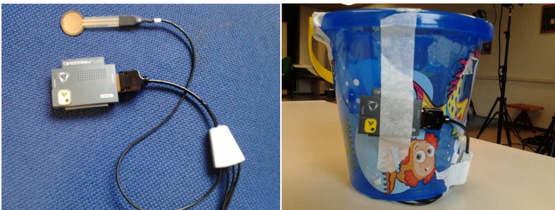
Figure 5.2.2: the pressure switch (on the left) was fixed at the bottom of the bucket, whereas the record unit (on the right) was attached outside the bucket
