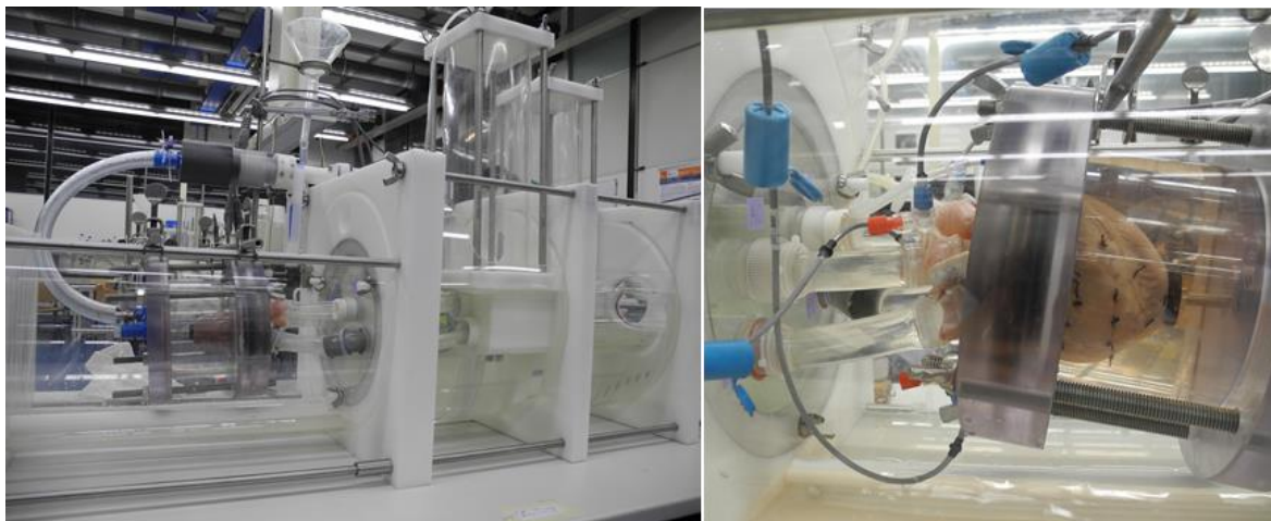
FIGURE 4. Pictures of the 4 chamber mock loop during one of the first experimental assessments that were carried out with passive hearts.
