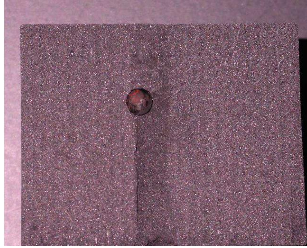
Figure 4.1: Low velocity impact on carbon foam sample [164].
