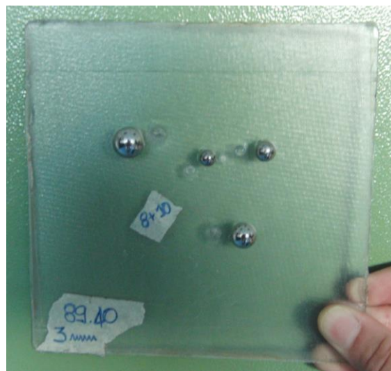
Figure 3.3: Example of specimen used in ballistic experiments.
