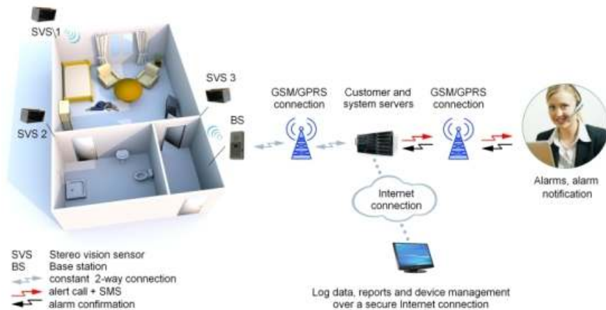
Figure 74. The project CARE to realize an intelligent monitoring and alarming system for independent living of elderly persons.
