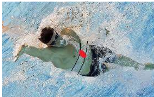
Figure 91. Swimmer with accelerometer on the central axis of the body just below the chest.
