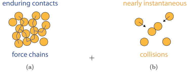
Figure 4.1.: Mechanisms of interaction between particles: enduring contacts among grains, which are involved in force chains (a), and inelastic collisions (b).
