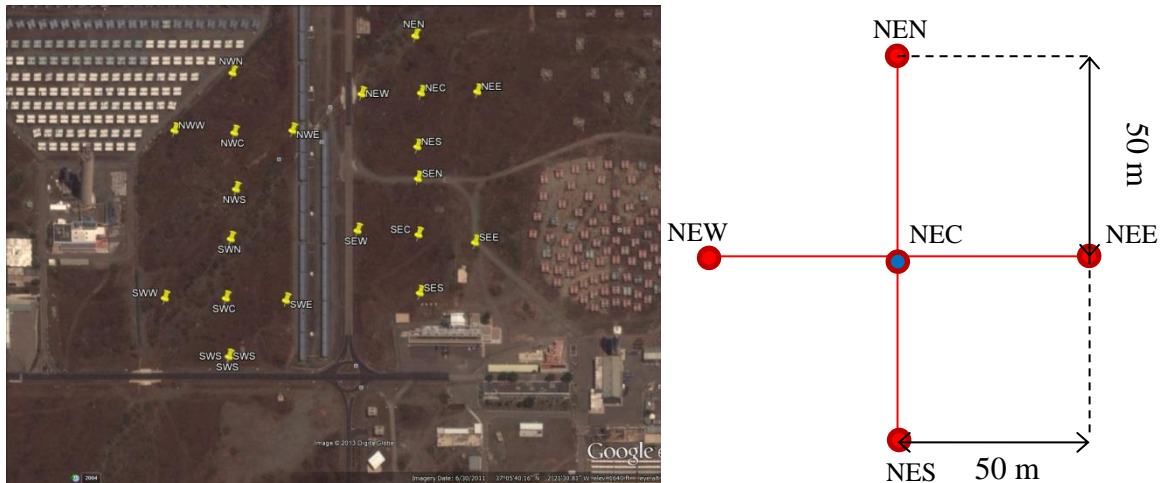
Figure 6.2 Installed GHI measurement grid at Plataforma de Almeria [6] (snapshot taken from Google Earth [9]) (coordinates: 37° 5' 30.12" N, 2° 21' 29.88" W) (left). Sketch of a diamond with the main length reported (right).
