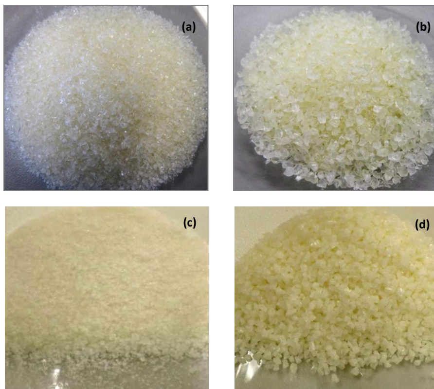
Figure 2.3. PAAH samples: MBA/EDA - d < 1\text{mm} (a), MBA/EDA - 1\text{mm} < d < 2\text{mm} (b), MBA/CYS - d < 1\text{mm} (c), MBA/CYS - 1\text{mm} < d < 2\text{mm} (d).
