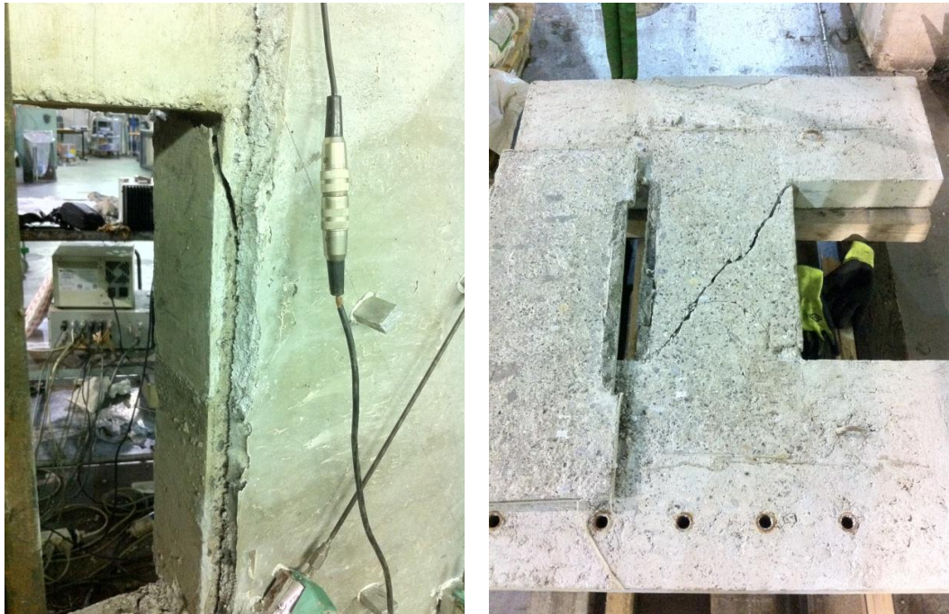
Figure 6.28 – Coupling beam repaired with HPFRCC at 1% pre-damage level – Failure of the beam
