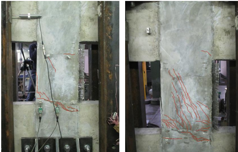
Figure 6.35 – Coupling beam strengthened with TRCC monotonic – Multiple cracks initiation and propagation under increased displacement
