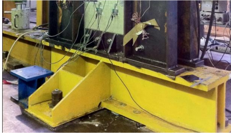
Figure 5.14 – Test rig fixed at base floor
