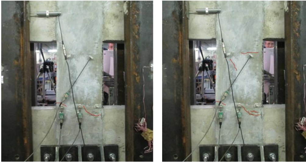
Figure 6.34 – Coupling beam strengthened with TRCC monotonic – Crack initiation and propagation under increased displacement
