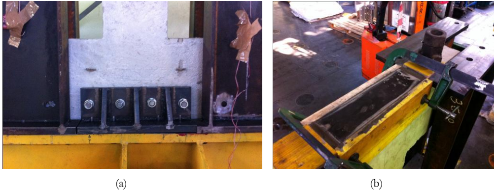
Figure A.7 – (a) fixing of specimen and (b) steel plate to guarantee planarity and provide sliding boundary condition
