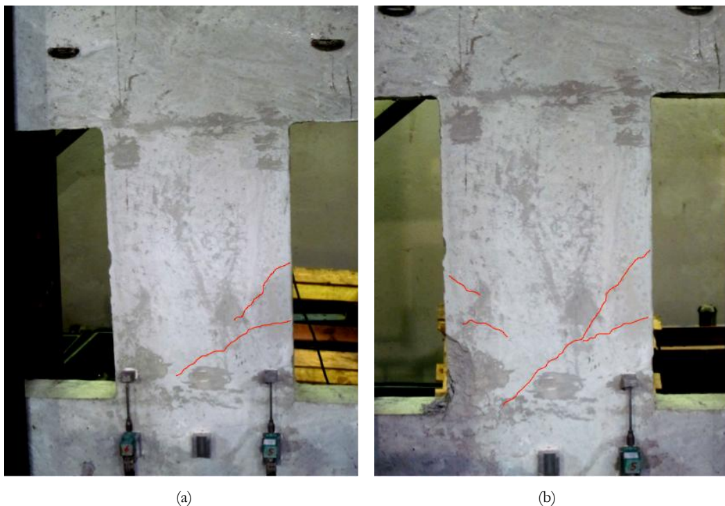
Figure 6.11 – Coupling beams with both longitudinal and transverse reinforcement under cyclic loading (a) at 1% drift and (b) at 1.5% drift
