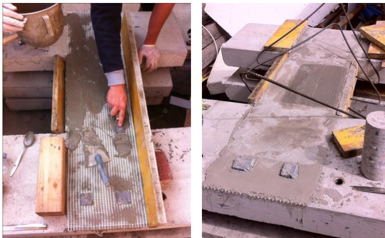
Figure 5.22 – Casting process for application of TRCC layer
