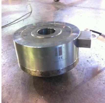
Figure A.9 – Compression load cell with capacity 400 kN
