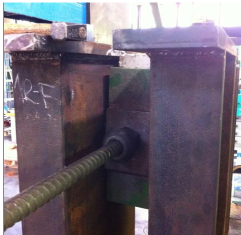
Figure A.6 – Load transfer from bar to the specimen
