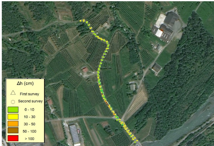
Figure 2.37: GNSS RTK points and absolute height differences with respect to PST-A DTM - area VT07.
