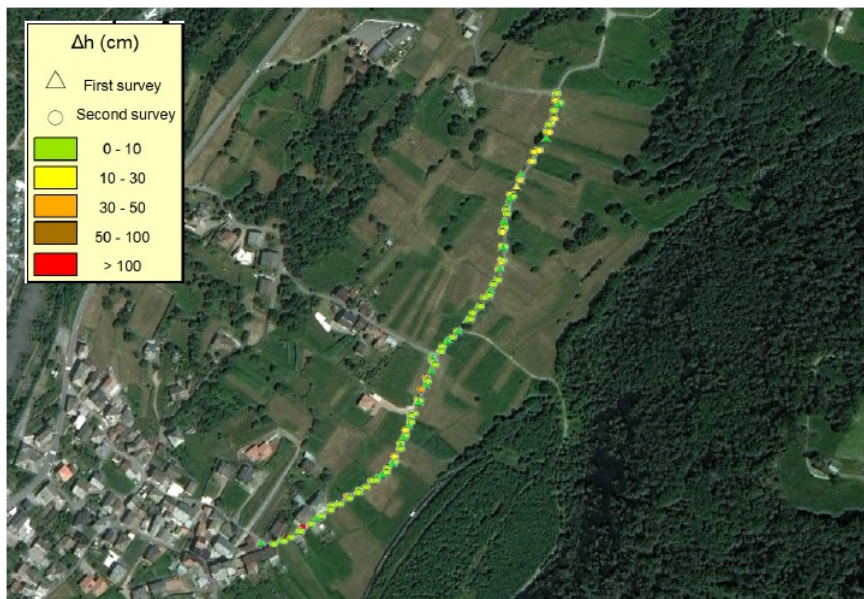
Figure 2.35: GNSS RTK points and absolute height differences with respect to PST-A LiDAR DTM - area VT09.
