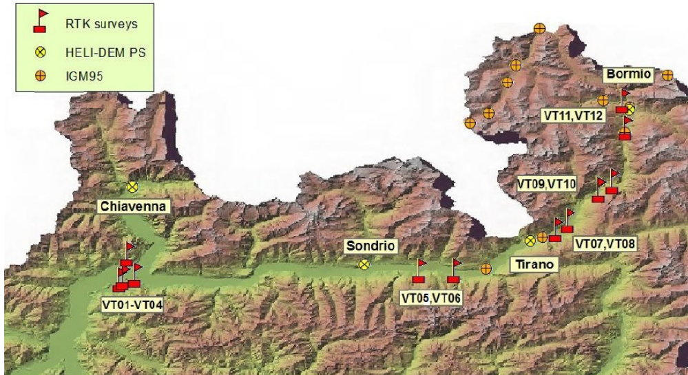
Figure 2.34: Selected areas in Valtellina Valley for the external validation of PST-A DTM with GNSS RTK surveys. In the map are indicated: the twelve areas selected for the RTK surveys (VT01-VT12), the Permanent Stations of the HELI-DEM GNSS network (HELI-DEM PS) and the IGM95 benchmarks.
