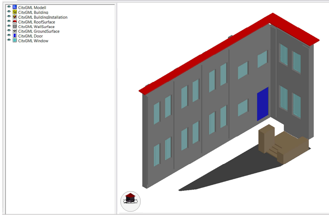
Fig. 5.15. Semantic reach model of the ‘Courtyard no.1’ in CityGML format. The model is visualized using the FZKViewer developed by the Karlsruhe Institut fur Technologie.
