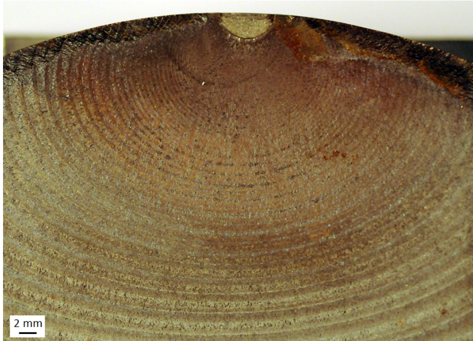
Figure 4.12: Fractography of the 3 mm notches, which developed in a big crack, at the end of the fatigue test
