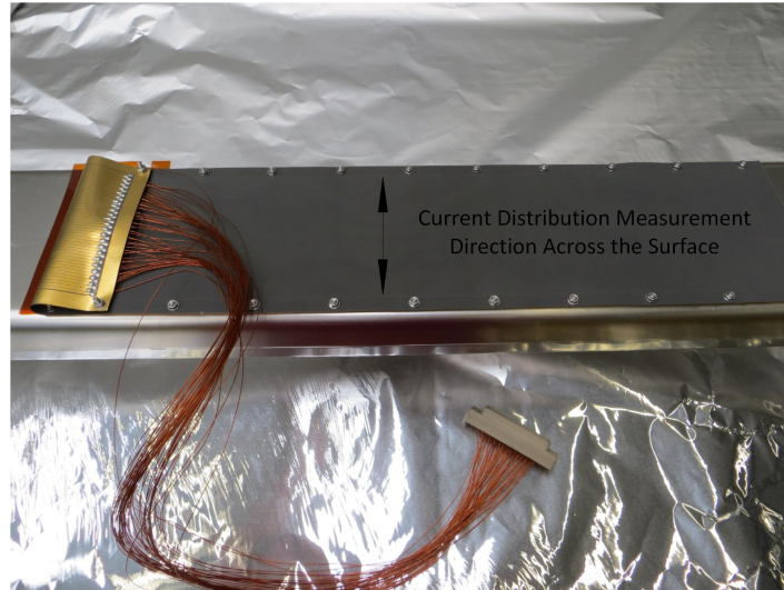
Figure 7.4: The current is measured along the chamber axis, its distribution can be resolved in transverse direction.
