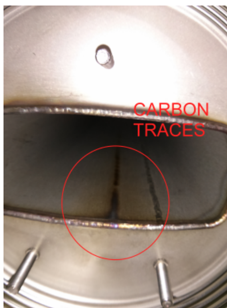
Figure 6.13: Residual traces of C on the MBB chamber after cleaning, induced by the beam exposure.
