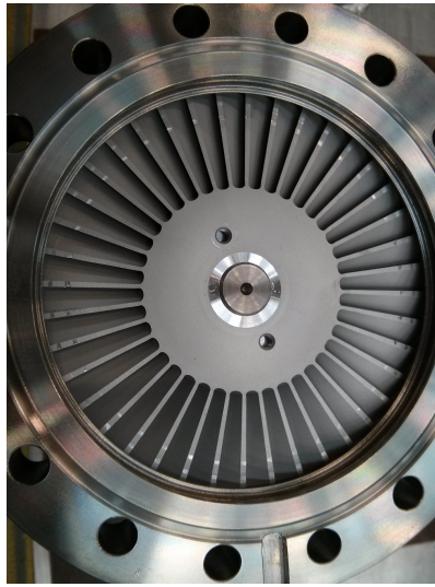
Figure 5.3: The old damaged turbomolecular pump of the pre-chamber. The blades are scratched, it influenced the pump performances and required to be changed.
