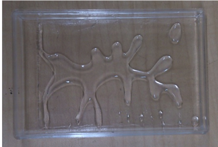
FIGURE 2.11: First attempt to create a thin PDMS membrane.
