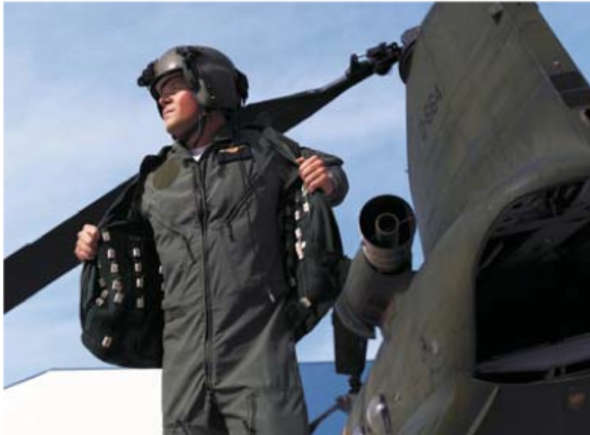
FIGURE 1.2: West equipped with vibrators for the spatial coding of positioning and bearing data [2].
