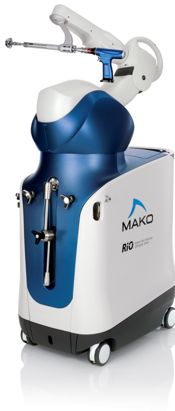
FIGURE 1.4: The Mako Rio™ is a surgeon interactive tactile surgical simulation platform that with a robotic arm allows the insertion and alignment of implants through a minimal incision.
