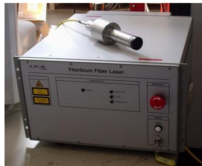
Figure 38. IPG YLP-1/100/50/50 Q-switched, long ns pulsed, 1 \mu\text{m} fibre laser source.
