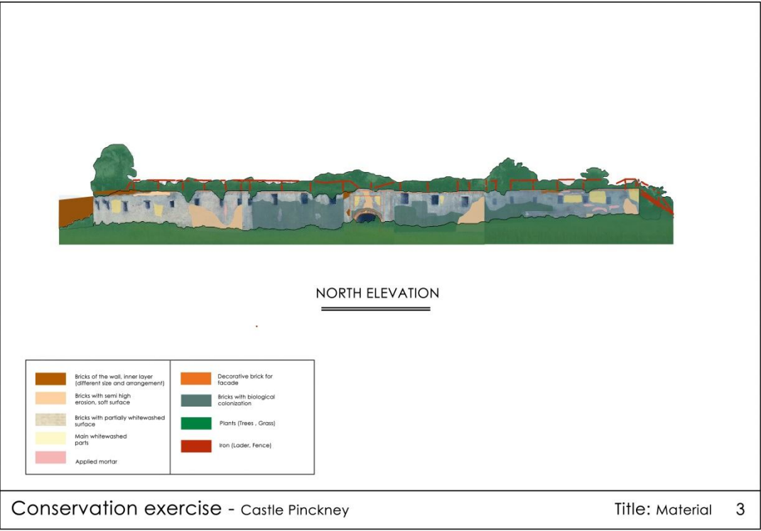
Figure 4.23, material of the Castle, North elevation
