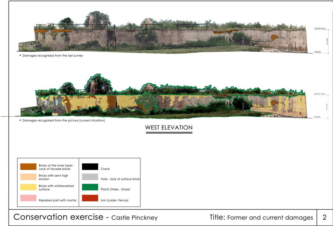
Figure 4.18, damages of the Castle, West elevation
