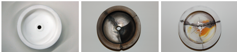
Figure 6.16: Plasma source backplate before (left) and after (center) about 40 hours of discontinuous plasma operation. The backplate is coated by sputtered steel and some cracks appeared due to thermal stress. On the right, the cleaned and repaired backplate is ready for another set of runs.
