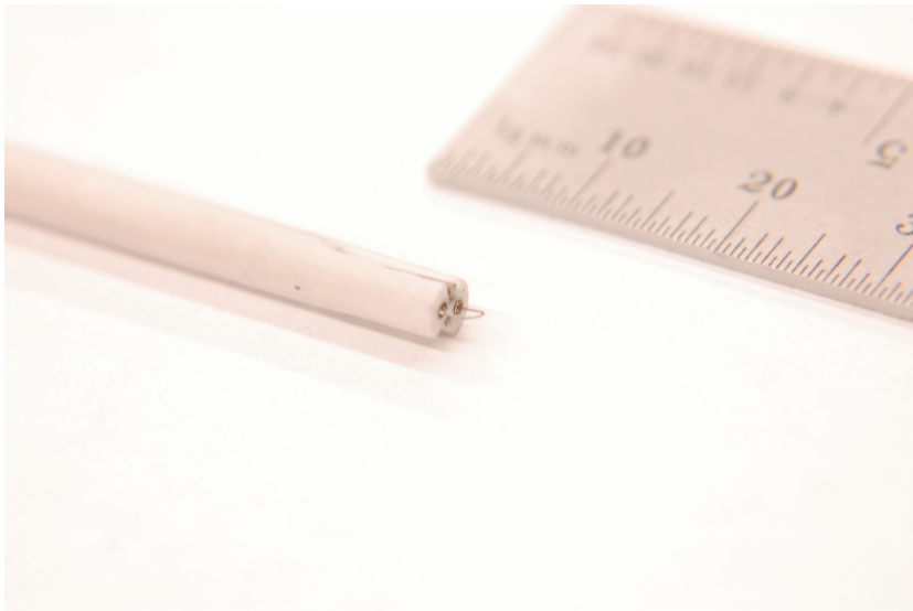
Figure 6.9: Combined Mach-emissive probe tip. The Mach probe is made of the two tungsten wires in the upper and lower sides, while the thin tungsten arch is the sensing surface of the emissive probe.
